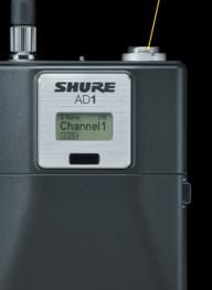
Backlit LCD with easy-to-navigate menu and controls
