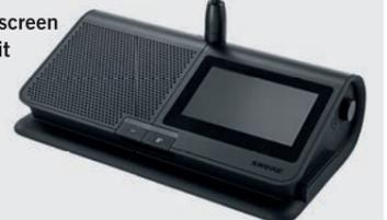
Portable conference unit which can be configured as a chairman or delegate unit. The unit features speak/function buttons, XLR gooseneck microphone connector, loudspeaker, two channel selectors and a touch screen for various functionality (microphone control, conference control, voting).
