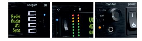
**Left:** Easily navigable grouped LCD menu **Middle:** RF mute switch and input level LED meter
