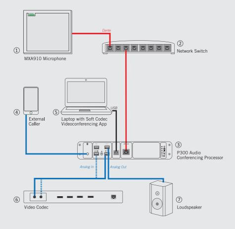
The P300 processes audio from the MXA910 Ceiling Array and sends it to the far end via the in-room video conference system. It also provides connectivity for USB and mobile devices at the table, allowing for easy collaboration with additional remote attendees. The P300's advanced DSP algorithms eliminate echo and noise to provide a high quality audio experience for natural and interactive conversations.
