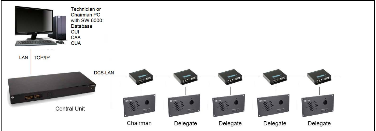
Figure 0-L DCS 6000 Digital Conference System with basic SW 6000 setup
